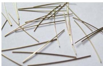
Figure 9: Straight Steel Fibers used
