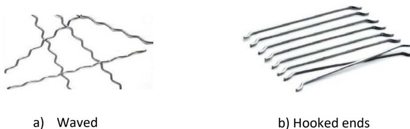
*Figure 4:* Types of steel fiber used
