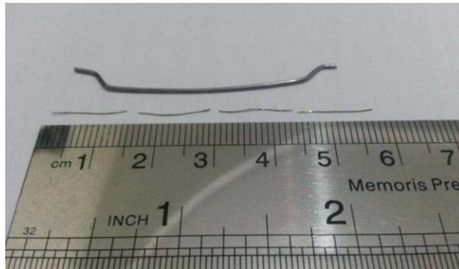
*Figure 10:* Micro and Macro Steel Fiber used
