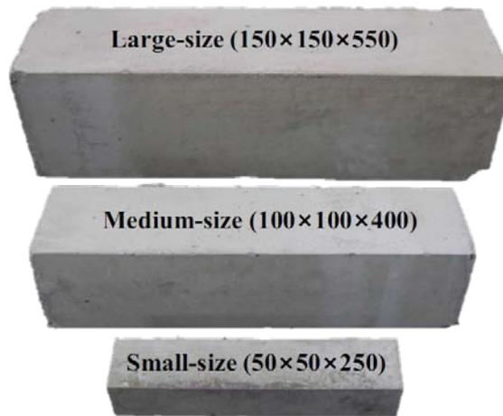
Figure 6: Geometry of Specimens Used (Units: Mm)
